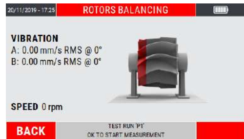
dual plane balancing test weight on plane "P1"
